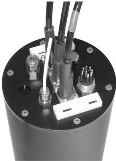
Connector endcap of a HydroRad-3
