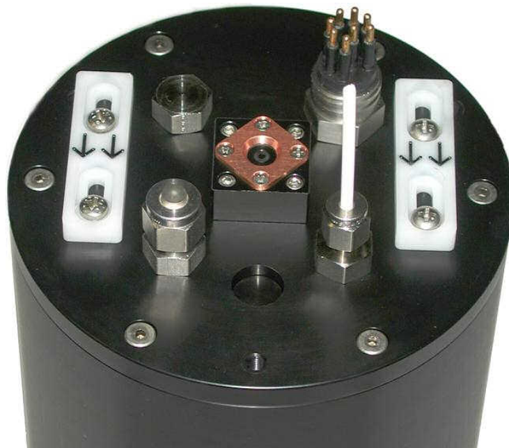
HydroRad-E2 Endcap with embedded Radiance Collector
